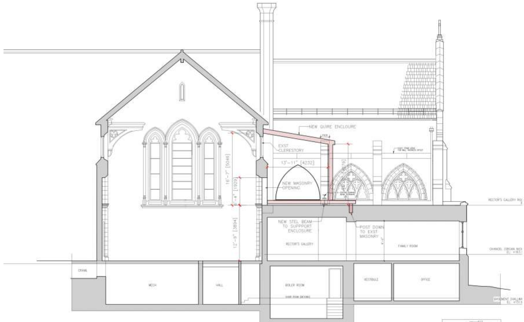
SECTION THRU QUIRE ENCLOSEURE LOOKING WEST 1/8" = 1'-0"
